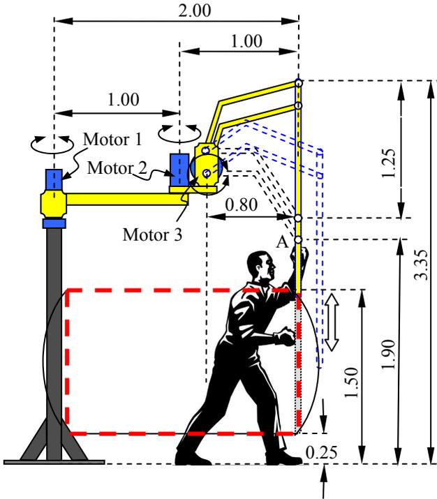
Fig. 1. Sketch of the main structure and dimensions of the power assists device (Units in meters).
