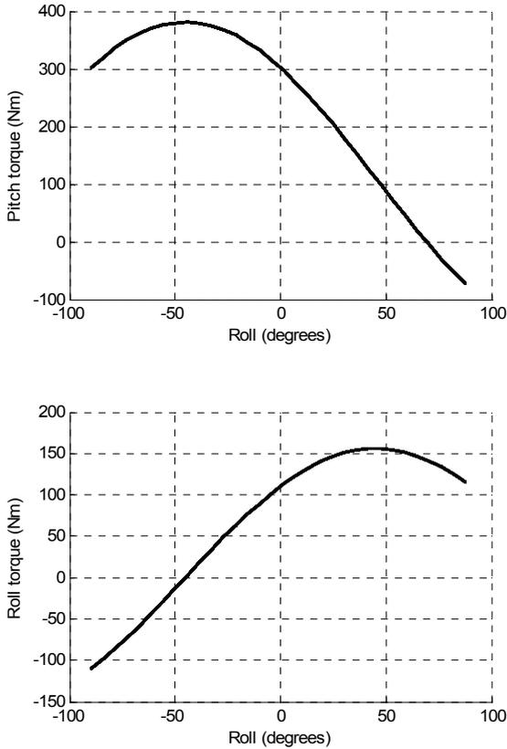
Fig. 6. Pitch and roll torques in the wrist joints as a function of the roll angle when the pitch angle is  $60^\circ$
