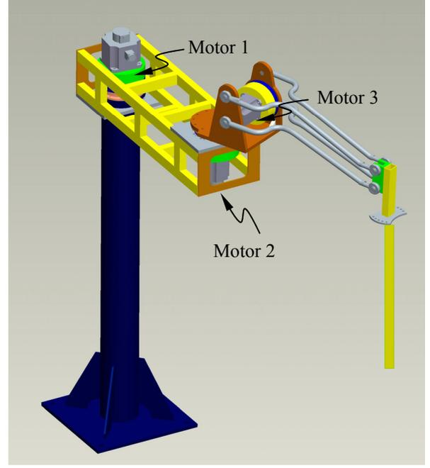
Fig. 4. Design of the Power Assist Device Arm
