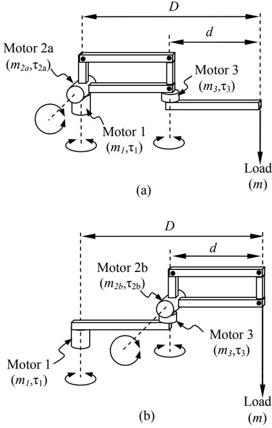
Fig. 3. (a) Traditional and (b) new PAD configuration
