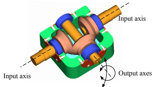
Fig. 7. Differential system of the wrist
