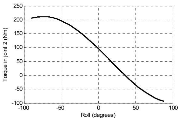
Fig. 8. Joint torques in a differential wrist as a function of the roll angle when the pitch angle is  $60^\circ$
