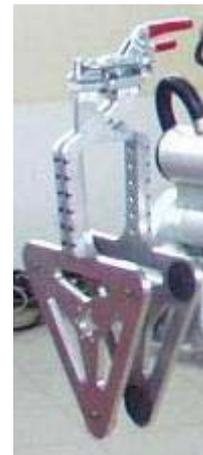
Figure 3. Grasping device for plaster panels
