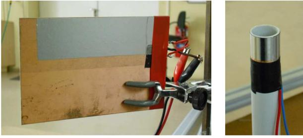
Fig. 2. Emitting (flat) and receiving (cylindrical) transducers fabricated with EMFi film.
