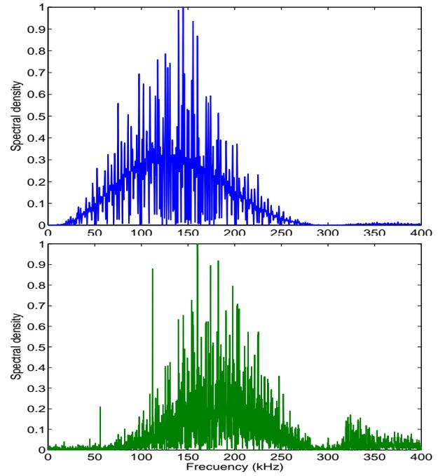
Fig. 6. Spectral densities of the emitted (top) and received (bottom) ultrasonic signals. The excitation signal is broadband, occupying a wide frequency range between 50 and 250 kHz. The spectral density is not seriously modified by transmission, although some higher gain at high frequencies can be appreciated, as well as the effect of the resonance at 325 kHz.
