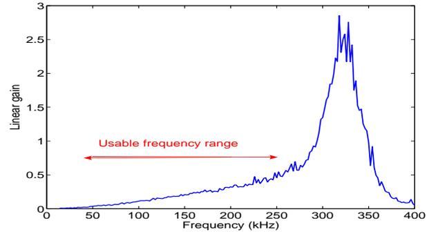
Fig. 4. Frequency response gain (linear plot) of the transducer system, and usable frequency range considered in this work.
