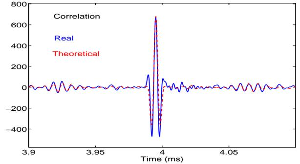
Fig. 7. Correlation of the received signal (blue) and comparison with theoretical correlation (red).
