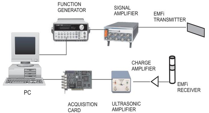
Fig. 3. Experimental setup for transmission and reception of CDMA ultrasonic signals with EMFi transducers.
