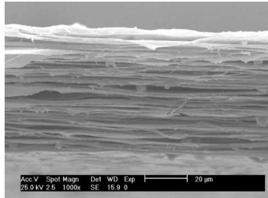
Fig. 1. Microphotography of the electromechanical film used in this paper, showing its internal, bubble-like structure.
