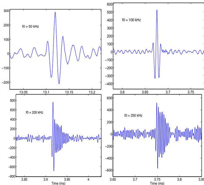
Fig. 8. Correlation of emitted codes at different central frequencies  $f_0$  (50, 100, 200 and 250 kHz). The amplitude of the correlation peak decreases at low frequencies and it starts to ring as we approach the resonance frequency of the film (325 kHz).
