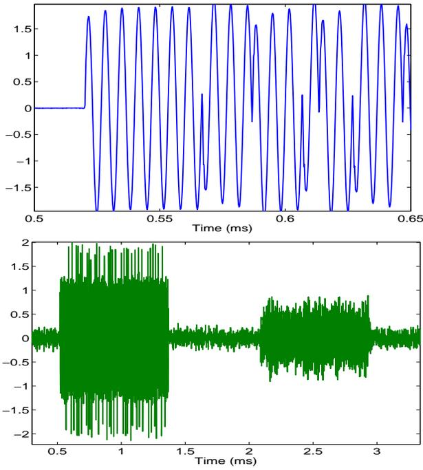
Fig. 5. (Top) Initial part of the excitation signal of the emitting transducer, showing phase changes of BPSK modulation (carrier frequency  $f_0 = 150$  kHz). (Bottom) received signal. The first part corresponds to electromagnetic coupling between emitter and receiver, the second part to the acoustic signal.
