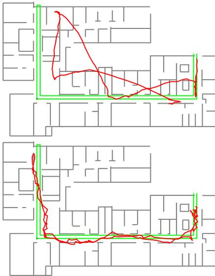
Fig. 8. Tracking of a simple C-shaped trajectory (green trace) by a particle filter with the RSS signals (without using PDR information) obtained from a network with only 4 anchor nodes (top); the calibrated network of Figure 6 (60 beacons, no anchor nodes) (bottom). Similar tracking performance is obtained with the calibrated network of Figure 7.
