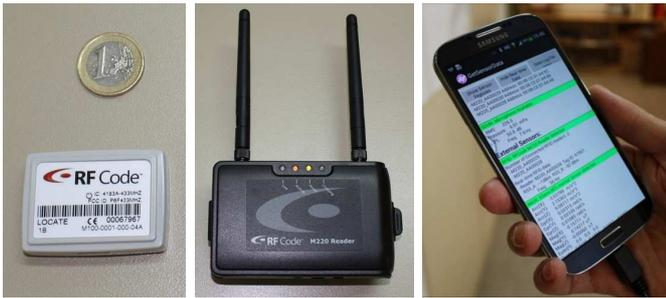
Fig. 3. Experimental device for demonstration of the autocalibration method, consisting of several active RFID tags, an RFID reader, and a smartphone.
