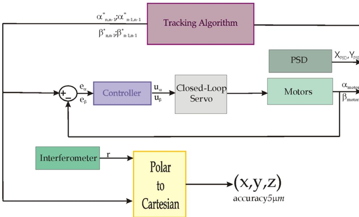
Figure 4. Layout of the Predictive Controller.
