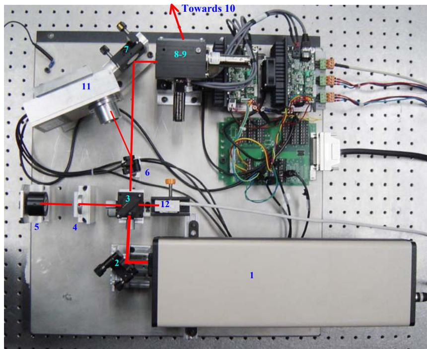
Fig. 2. An image of the different optical elements in the optical measurement system.
