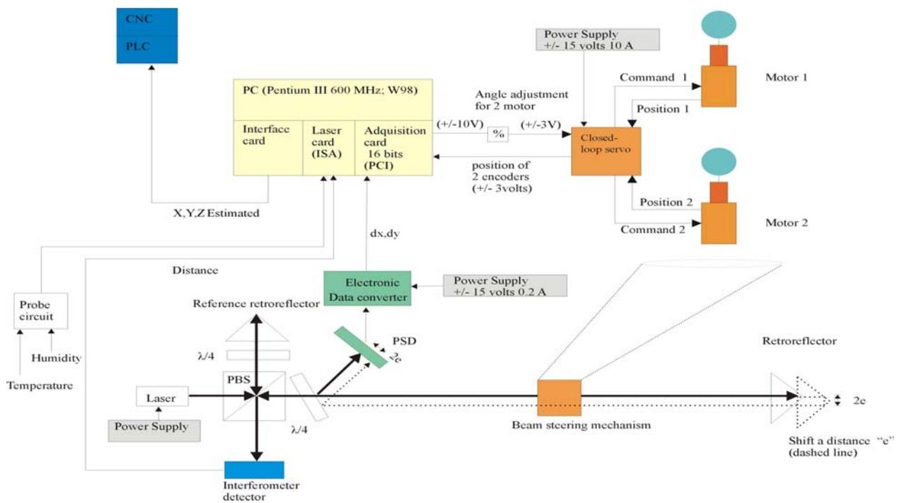
Figure 3: Layout of the optical 3D measuring system.
