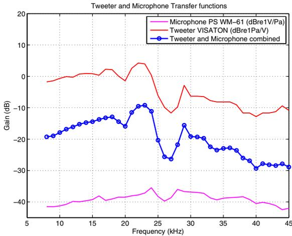
Fig. 2. MICROPHONE AND TWEETER FREQUENCY RESPONSE
