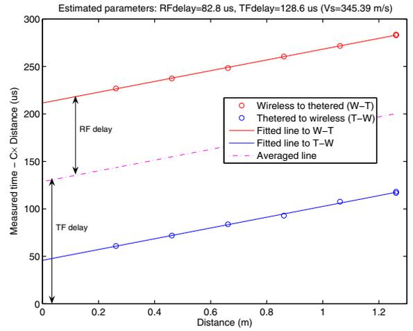
Fig. 4. LINEAR REGRESSION OF DISTANCE MEASUREMENTS TAKEN BETWEEN WIRELESS AND TETHERED NODES
