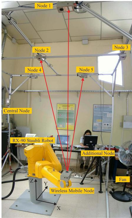
Fig. 5. ROBOTIC CELL EMPLOYED FOR SYSTEM EVALUATION
