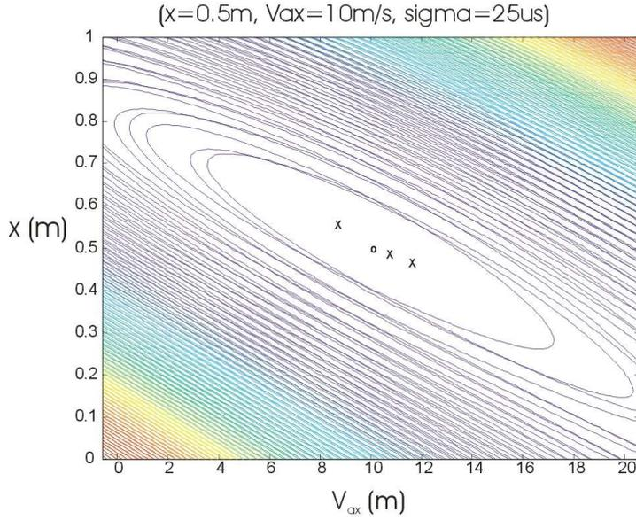
**Figure 12:** Multilateration cost-function contour graph for two dimensions ( $x$  and  $V_{ax}$ ). Central circle indicates real values ( $x = 5$  m and  $V_{ax} = 10$  m/s); Crosses indicates several noisy estimates both in position and air speed.
