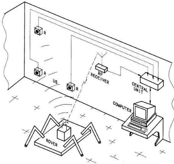
**Figure 2:** Localization system for Rimho walking robot
