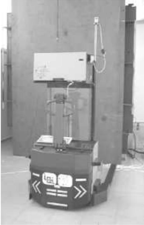
**Figure 3:** Automated pallet truck for 'Intelligent Warehouses'. Omnidirectional ultrasonic receiver on the upper tip of the vertical post
