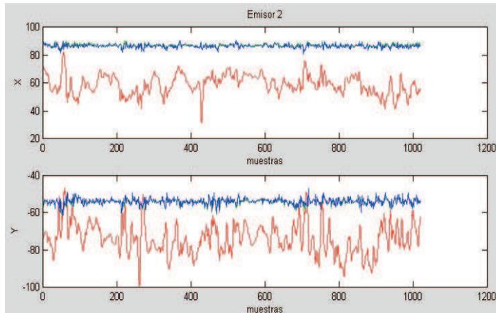
**Figure 13:** (Red) X and Y estimations under a wind-flow varying between calm condition to 5 m/s speed, which suffer from errors up to 5 cm ; (Blue) Same case but using the compensation method, a moderate to good compensation (1 cm error still remains) is obtained for this case where reference station is 1 m apart from point of interest
