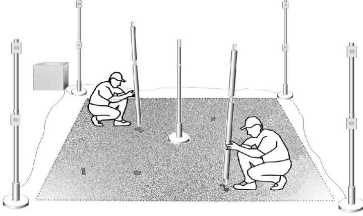
**Figure 11:** Designed ultrasound localization system for archaeological applications
