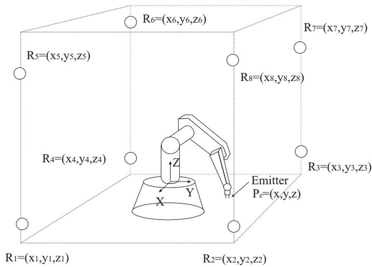
**Figure 8:** Redundant 8 receiver configuration for Kaylite project
