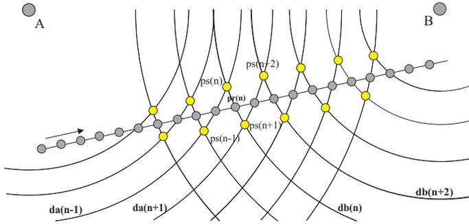
**Figure 5:** Error caused by non-simultaneous measurement of TOA from beacon A and B. Gray spots indicate the real straight trajectory followed by the robot; Yellow spots are the erroneous estimations, before applying the proposed correction, that zig-zag at both sides of the real trajectory.
