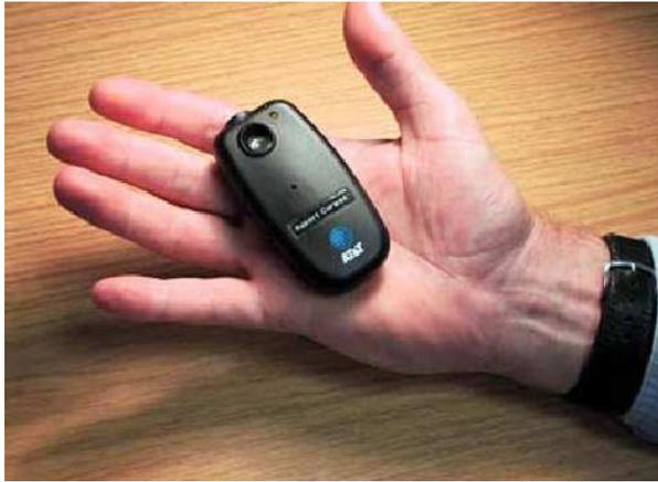
**Figure 1:** Ultrasonic mobile 'Bat' device to be carried on the person's chest, as part of the AT&T 'Active Bat' location system
