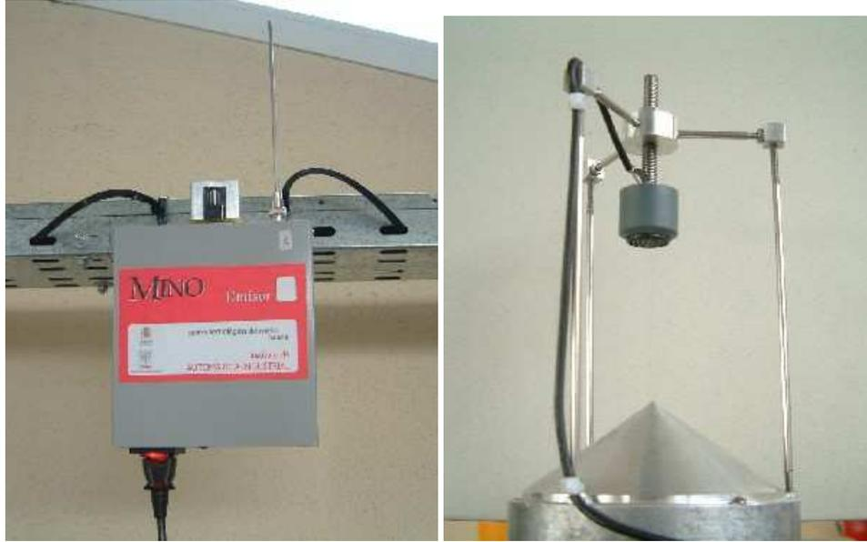
**Figure 6:** Emitter and receiver transducers in the Mino system.
