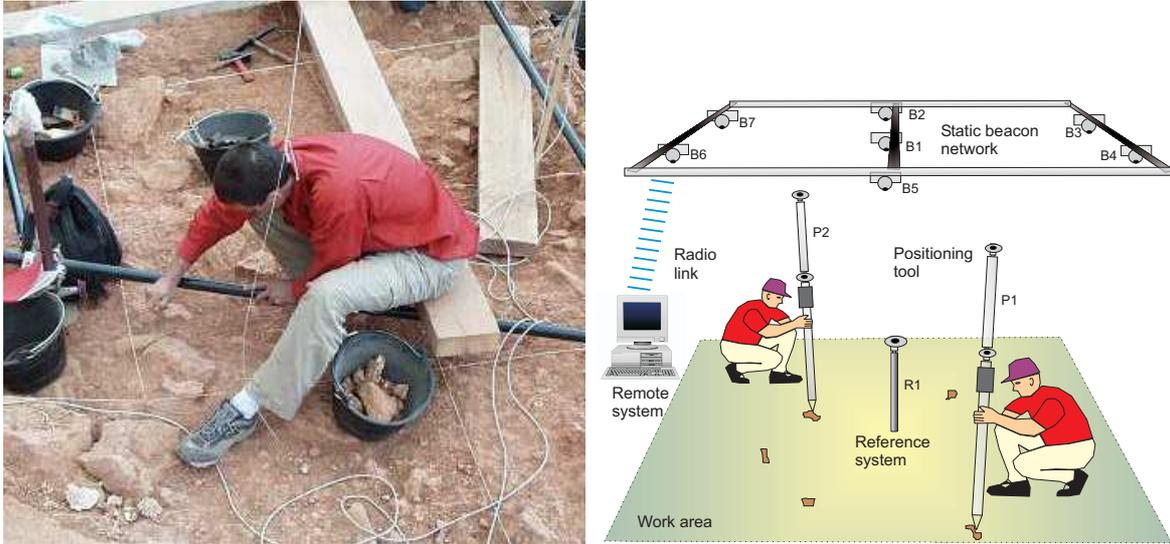
**Figure 4:** Manual positioning of pieces in archaeological findings and the system developed at the IAI for assistance and automatization of the task.
