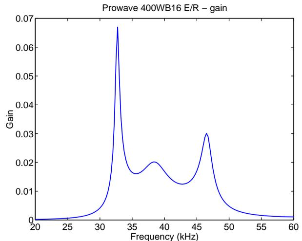
**Figure 7:** Frequency response gain of the transducers of figure 6.
