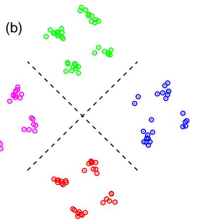
**Figure 13:** (a) Transmission signal, including the header and a 256 bits QPSK modulated message; (b) symbol constellation obtained after demodulation.
