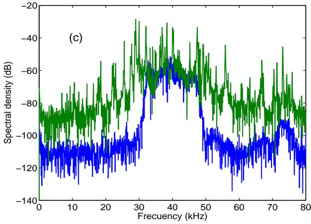
**Figure 12:** Signal detection with impulsive noise: (a) received signal, (b) correlation, and (c) spectrum of the signal (blue) and the noise (green).
