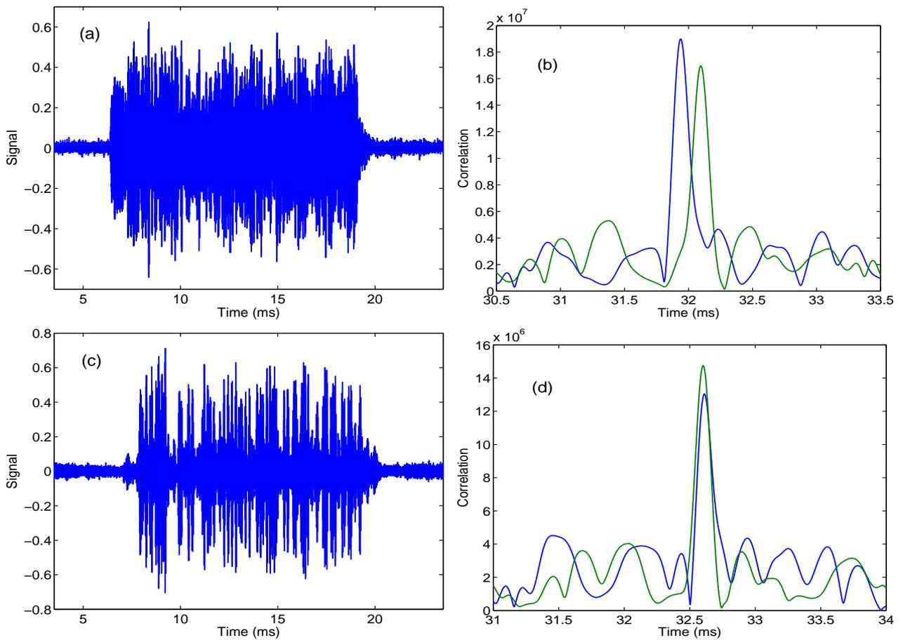
**Figure 9:** Echo separation capability of two orthogonal codes. In (a) the emitting transducers are separated 53 mm (156 μs); the correlations with each code are shown in (b). In (c) and (d) the transducer separation is 3 mm (8.7 μs).
