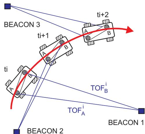
**Figure 1:** Tracking of a mobile vehicle with an ultrasonic positioning system.
