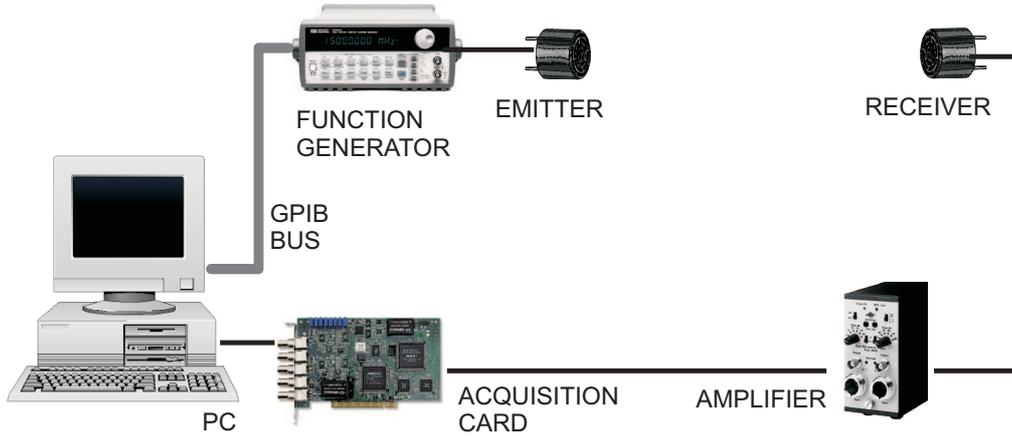
**Figure 6:** Experimental setup for the modulation and codification of ultrasonic signals.
