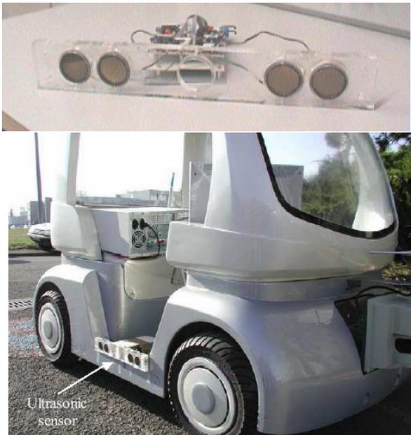
**Figure 5:** Four transducers (2T/4R) sensor structure employed at the Universidad de Alcalá, and its application for SLAM in a CyCab vehicle.
