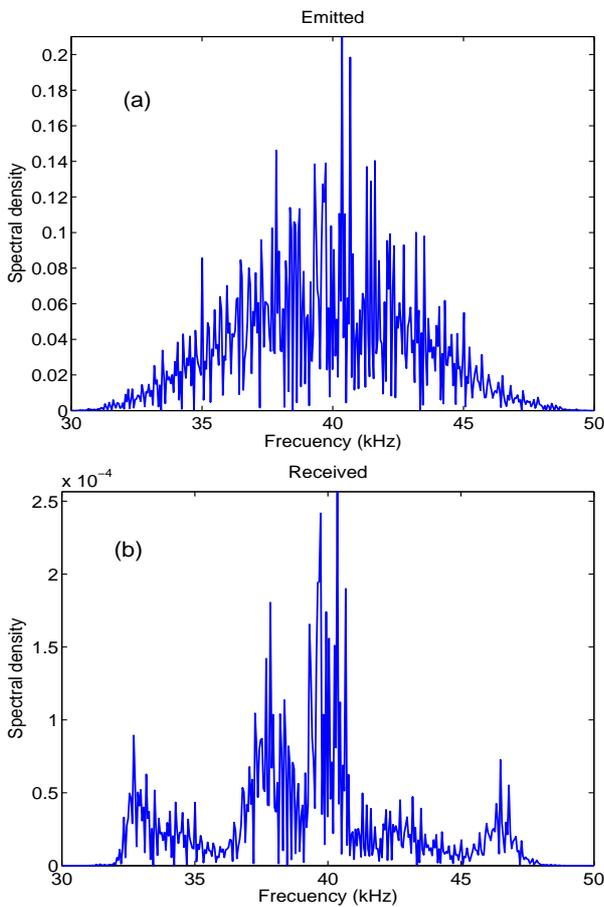
**Figure 8:** Spectral density of a modulated Gold code: (a) as emitted; (b) after reception.
