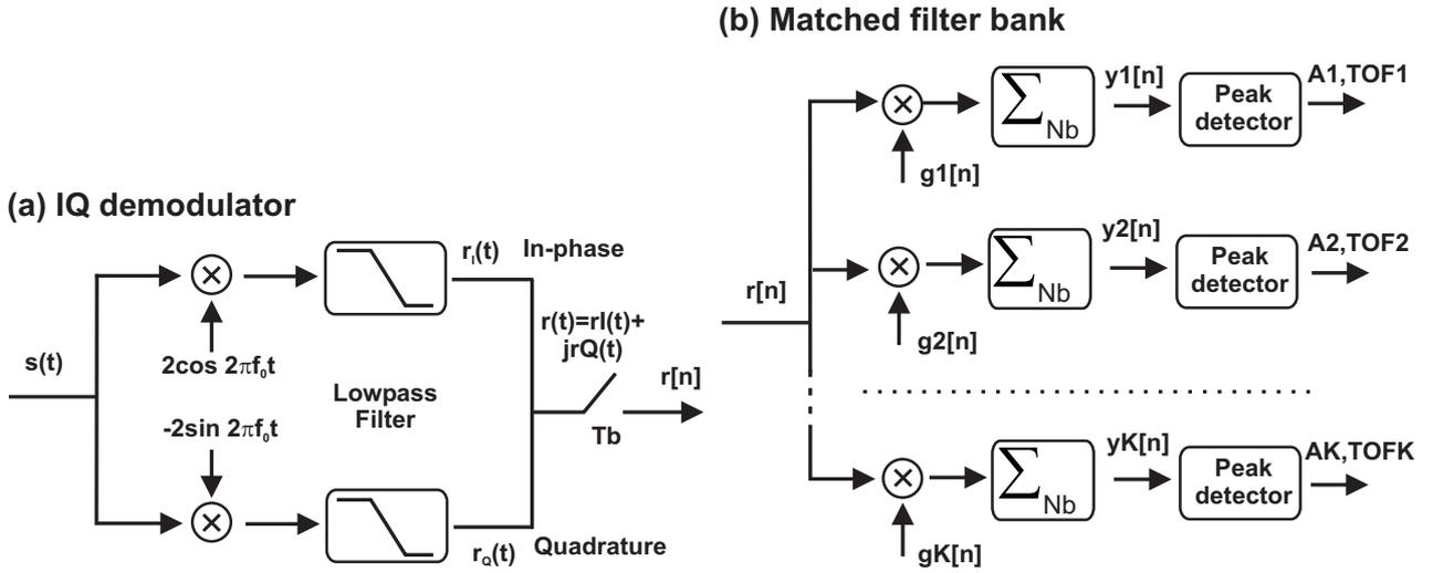
**Figure 3:** Processing stages of a CDMA system: (a) Inphase-quadrature (IQ) demodulator used to compute the complex envelope or baseband representation of the ultrasonic signal; (b) Correlator bank to detect the different users.
