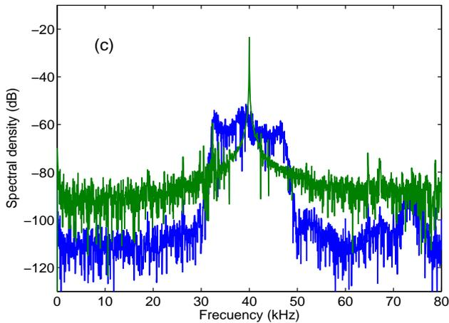
**Figure 11:** Signal detection with narrowband noise: (a) received signal, (b) correlation and (c) spectrum of the signal (blue) and the noise (green).
