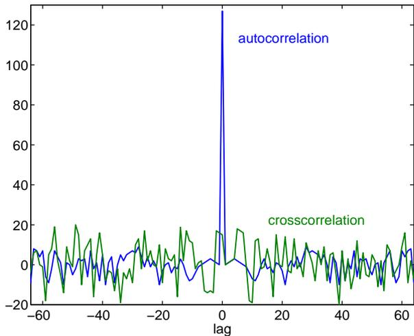
**Figure 2:** Autocorrelation (blue) and cross-correlation (green) of two 127 bits long Gold codes.
