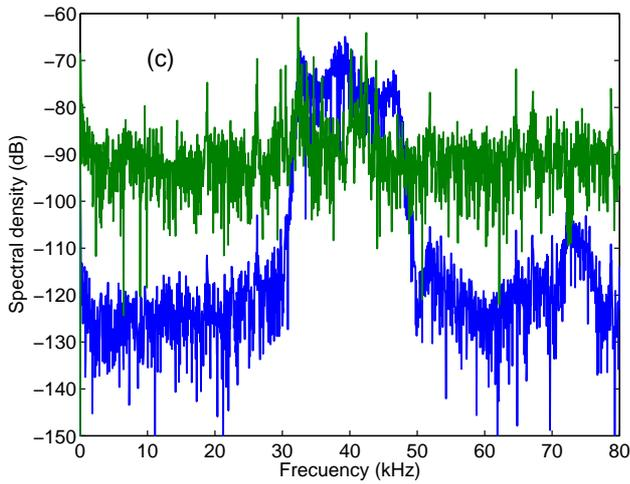
**Figure 10:** Signal detection for low SNR: (a) received signal, (b) correlation, and (c) spectrum of the signal (blue) and the noise (green).
