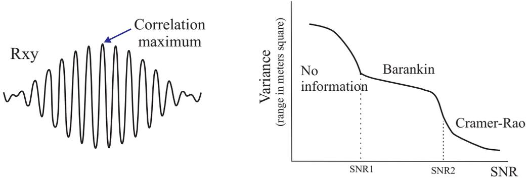
**Figure 6:** (left) result of correlating the received signal with the stored reference; (right) Regions where estimation variance changes with SNR at certain thresholds. This thresholds change with bandwidth, duration and frequency of signals
