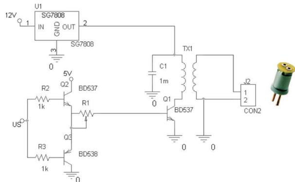
**Figure 5:** Electronic circuit for ultrasonic PVDF excitation
