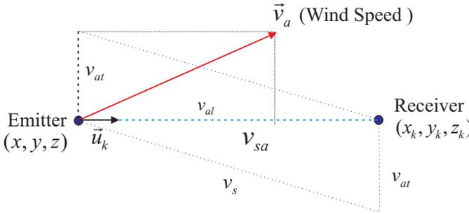
**Figure 7:** Air flow components  $\vec{v}_a = \{v_{al}, v_{at}\}$  with respect to the emission-reception axis
