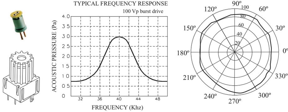
**Figure 4:** Omnidirectional PVDF transducer used as emitter. (left) PVDF film is shaped in a cylindrical holding and protected with an external grid; (center) Its frequency response around 40 kHz; (right) horizontal ultrasonic emission lobe
