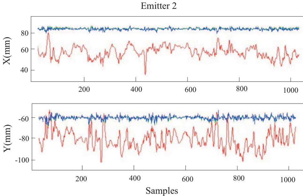
**Figure 9:** (Red) X and Y estimations under a wind-flow varying between calm condition to 5 m/s speed, which suffer from errors up to 5 cm ; (Blue) Same case but using the compensation method, a moderate to good compensation (1 cm error still remains) is obtained for this case where reference station is 1 m apart from point of interest
