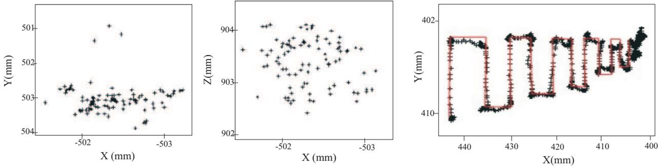
**Figure 8:** (left-middle) Accuracy and repeatability indoors tests showing the dispersion in 3D position estimation; (right) Resolution indoors tests performed following a predefined increasing-size pulse-like path
