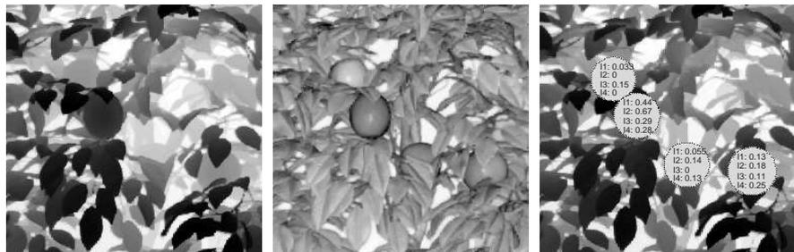
Figure 10: Fruit recognition example. From left to right: scene photo, range, reflectance images and detections found.
