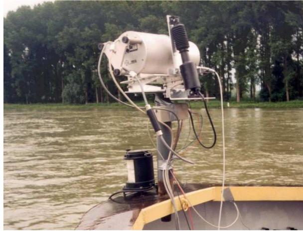
Fig. 3. Picture of the ladar system on the bow of a vessel in navigation trials.
